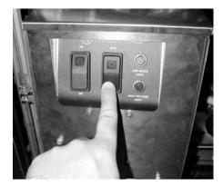
2. Energize heating circuit to pre-heat unit.
